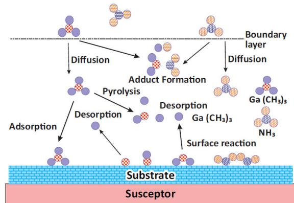
Fig. 1: Schematic of different processes in MOVPE.
