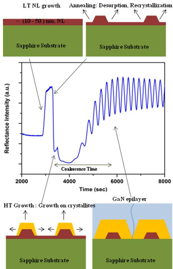
Fig. 4: In-situ reflectance trace along with growth steps (Sample-B).
