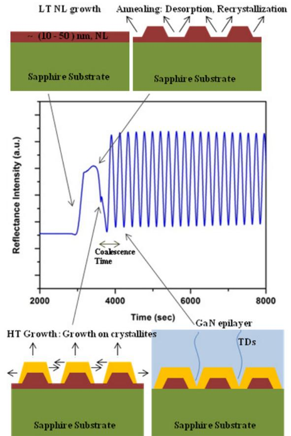
Fig. 3: In-situ reflectance trace along with growth steps (Sample-A).
