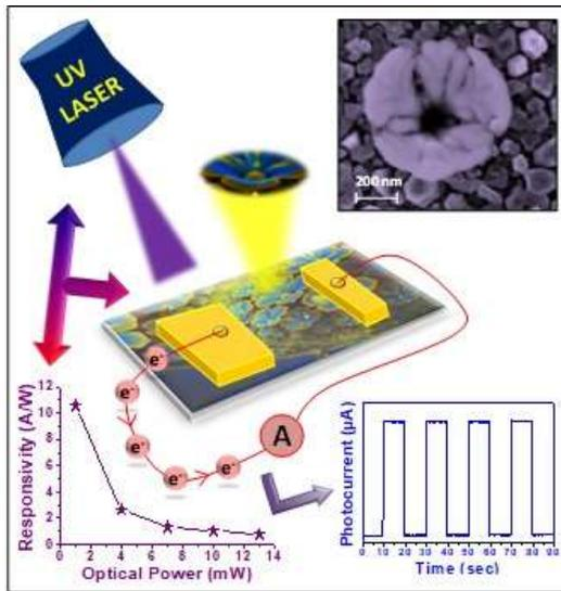
Figure 2: A layout of the GaN Nanoflowers based UV illuminated photodetection device yielding stable response and its dependence of responsivity with optical power showing highest value at 1 mW.
