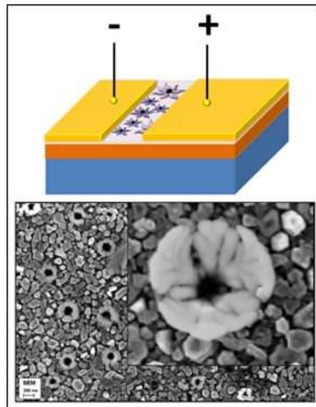
Figure 1: Schematic diagram of fabricated device and Field Emission Secondary Electron Microscopic images of epitaxially grown GaN NFs.
