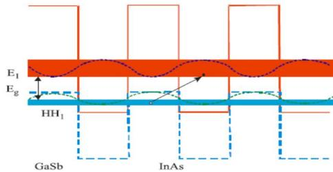
**Fig.3. Band diagram of GaSb-InAs T2SL structure**
