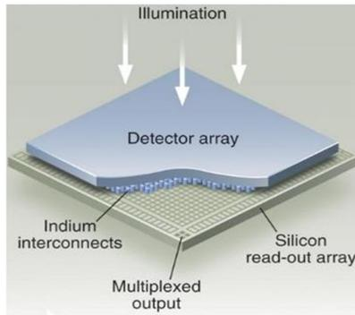
**Fig.1. Configuration of hybrid IR Focal Plane Array detector**
